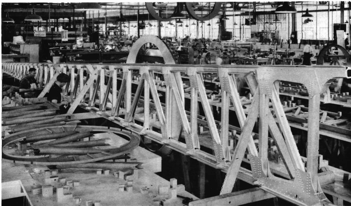
Wing-spar for a Boeing Clipper. This shiny assembly is the front spar for the main left-hand wing-panel for a Boeing 314 Clipper. The ring in the center of the picture marks the location of the outboard engine nacelle. Both the upper and lower spar chords are square steel tubes.
