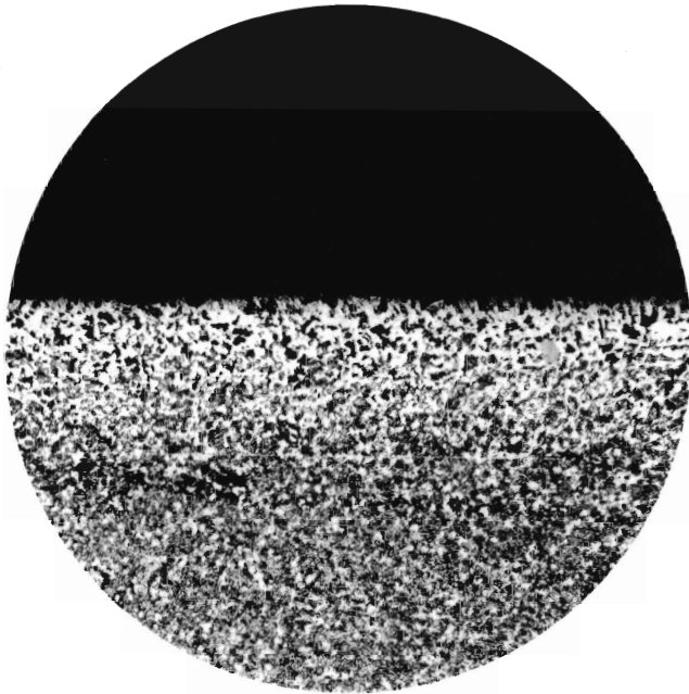
Reproduction of decarburized surface of X4130 normalized steel tubing. (Magnification X100.)
