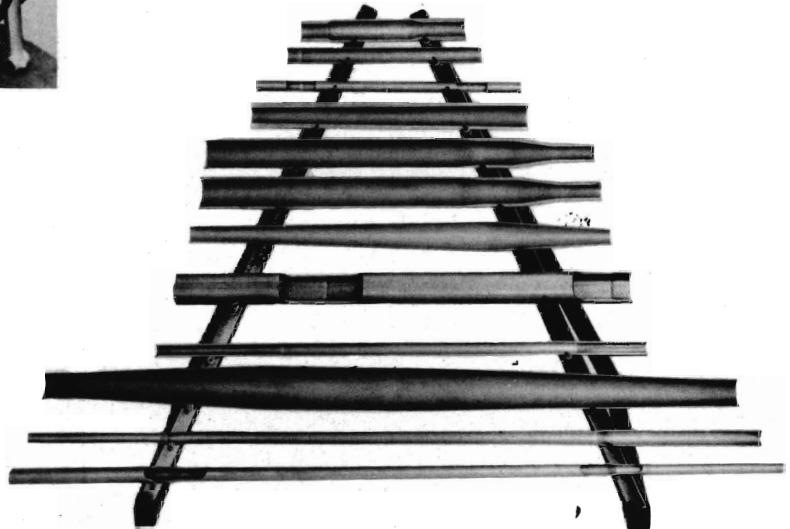
Shown above is a small selection of various tapered, step-tapered, swaged and formed tubes. These examples are merely representative of some of the special tubing being produced for the aircraft industry.
