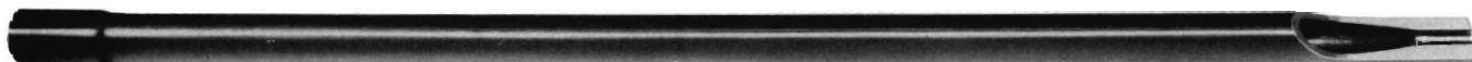
This tube has an outside upset on one end and an inside upset on the other end. Due to relatively light wall for major length of tube, this particular piece has been produced by a combination of swaging and machining.
