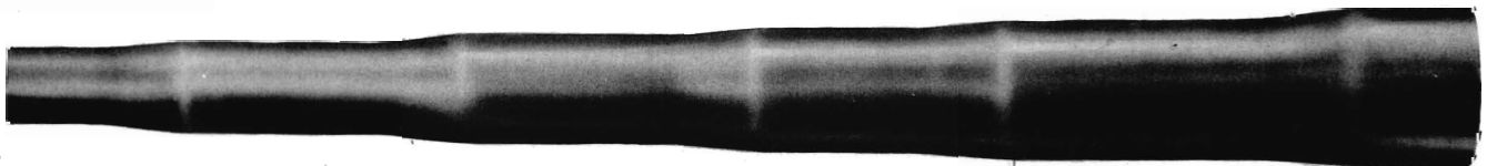
\frac{5}{8} " O.D. x .156" wall tapered in five steps to 2\frac{1}{2} " O.D. x .100" wall. Note the long, smooth tapers at each step.
