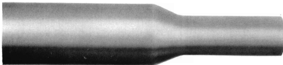
3\frac{3}{4} " O.D. x .049" wall tapered to 2\frac{3}{8} " O.D. x .049" wall for torque tube. This large reduction at end of torque tubes greatly reduces the size and weight of the required fittings.
