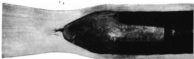
Figure 2. Section of billet removed from between the piercing rolls and still retaining the piercing plug. Note rupture of steel in front of plug.
