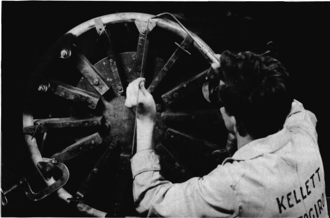
Gas Welding Engine Mount forgings to tubular ring.
