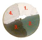
After shooting a "blank" to calibrate the spectrometer, one of the painted areas on the disk was placed between the light source and the sensor. The light source flashes on (2 seconds for our test) and the sensor picks-up any energy that makes it through the paint.
